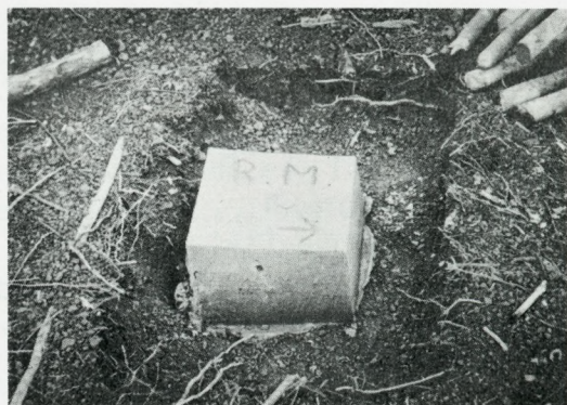
Completed reference monument at "Tiger"
